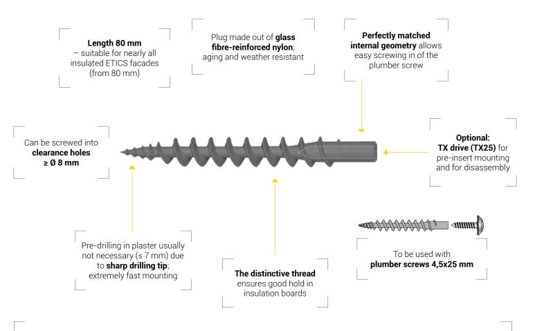
The Insulation screw plug IPSD 80 is perfectly suitable for direct fastening into insulation materials without a thermal bridge of wall connection profiles and other light duty fixings like motion detectors. Suitable insulation materials: Styrofoam boards, hard foam boards, polystyrene boards, wood fibre boards, suitable to a limited extent: mineral wool boards
